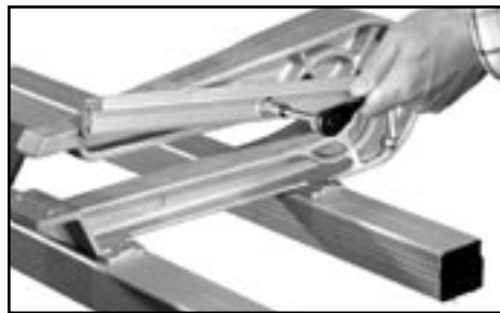
7 Remove Pivot Arm Remove Pivot Arms and springs and replace the Shoe Casting. When replacing, make sure all fasteners are tight
