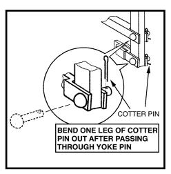
Insert Cotter Pins through holes in ends of both Yoke Pins. Bend one leg of each cotter pin forward to secure Yoke Pin.
