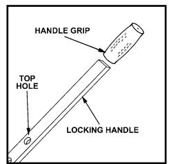
Remove Locking Handle and Handle Grip from parts bag. Press Grip over end of Locking Handle and slide down until Grip is firmly seated. Remove rest of parts from bag and proceed to next step.
