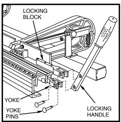
2Insert bottom end of Locking Handle into the bottom Yoke on right side of Port-O-Brake.® Align holes and insert Yoke Pin. Align top hole in Handle with holes in Locking Block of Slide Bar and insert second Yoke Pin.
