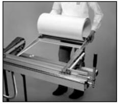
Hooks on and detaches in seconds. Allows you to roll out and cut coil squarely to your exact length.
