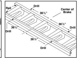
**2**Invert Brake. From center of Brake, measure outward along each rail 36<sup>1</sup>/<sub>2</sub>" and drill one pilot hole in center of each rail using an 11/64" drill bit.
