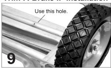
To install wheel kit on Trim-A-Brake II® models, use inner cotter pin hole. Trim excess axle shaft using a hacksaw.
