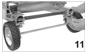
Slide the screw heads into the slots on each side. With the ends of the brackets flush to the ends of the base rail, tighten all hex nuts firmly in place with a 7/16" wrench.
