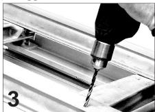
Using the bit provided, drill all 4 holes. Use a center punch to ensure accuracy of holes.
