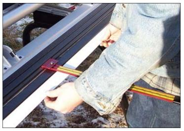
**Transporting your brake** - aside from clamping scrap materials in your brake to prevent internal scratching, it is a good idea to remove your slitter while traveling. This is accomplished by pulling the spring loaded pin and sliding the slitter off the brake slitter track.
