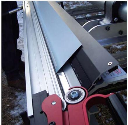
**Hemming** - Lock brake after inserting to desired depth. Bend to the max. Remove. Re-lock brake. Insert between stainless edge and rubber strip. Pull on handle to crush angle flat.
