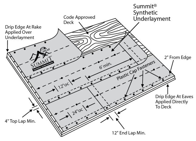
Summit 180 shall be applied to properly ventilated, building code approved roof decks. Before getting started, be sure the roof deck is clean, solid, properly fastened, and free of voids and/or damages.
