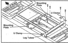
Set legs onto Brake with leg tubes near drilled pilot holes. Place "U" clamps over leg tubes, align holes and install sheet metal screws. Drill remaining holes through clamps and install screws. Install screws also in mounting plates as shown.
