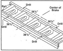
2 Invert Brake. From center of Brake, measure outward along each rail 361/2" and drill one pilot hole in center of each rail using an 11/64" drill bit.
