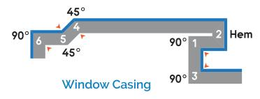
Pro Tip: The 45 degree bends on the left side of this example can also be shaped by using the Van Mark TrimFormer.
