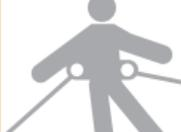
**Work Positioning:** Hitch Clips™ may be used in Work Positioning applications. Work Positioning systems allow a worker to be supported while in suspension and work freely with both hands. Structure must withstand loads applied in the directions permitted by the system of at least 3,000 lbs. Maximum allowable free fall is 2'. Applicable D-rings: Side, Shoulder.
