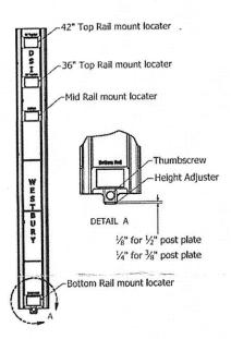
Height adjuster will allow template to be used on both 3/8" and 1/2" post plates to maintain 2" spacing between bottom rail and ground level.
