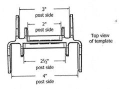
Template will locate top rail, mid rail and bottom rail mounts on post for 36" and 42" tall aluminum railing sections.
